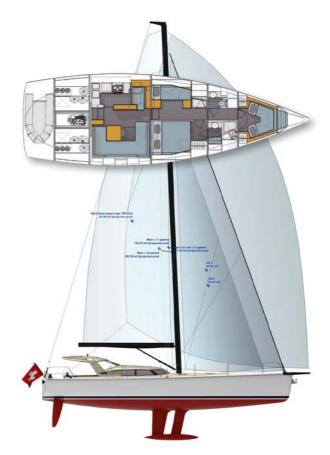
**LOA** 49' Beam 15'10" **Draft** 7'8" (std) Displacement 25,794 lbs (loaded) Ballast 8,487 lbs Sail Area 1,386 sq ft (main and 104% jib) **Engine** Volvo D2-75 Designer Marine Designs **Builder** Pegasus Yachts Price €1,250,000 (U.S. \$1,426,000 as of press time)
